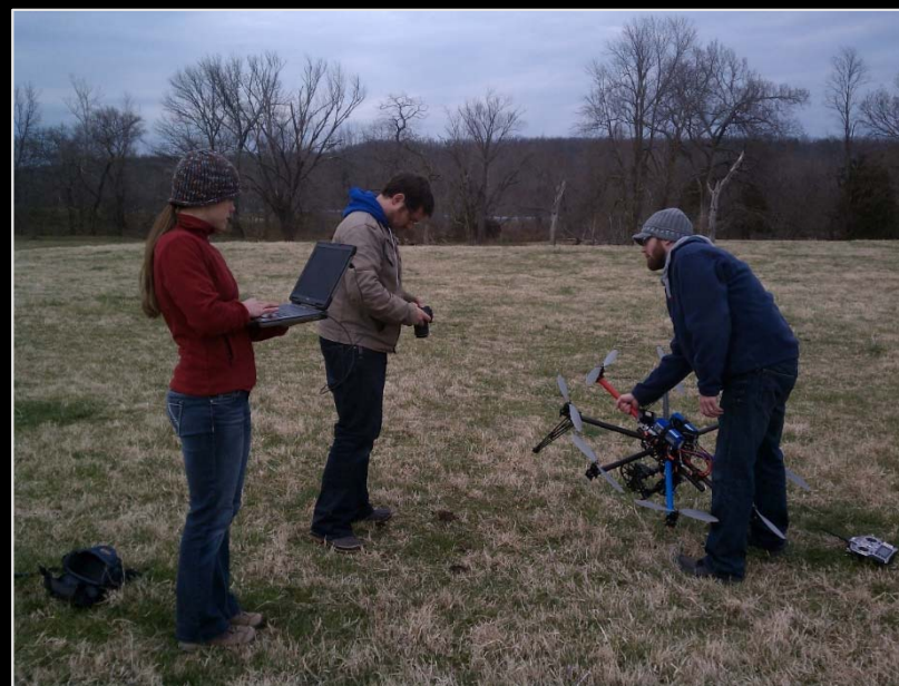
Cinestar 8 octocopter with Nikon D600 DSLR camera with a 35.9x24.0 mm sensor
