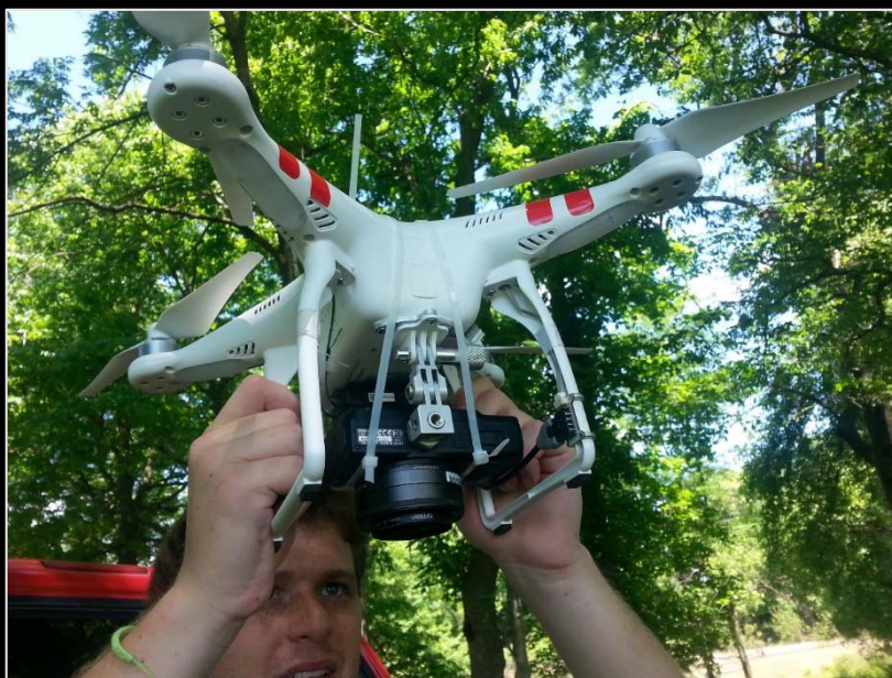
DJI Phantom 2 quadcopter with Canon EOS M camera with 22 mm lens
